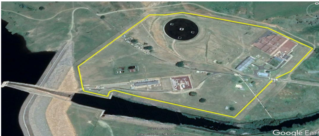
Figure 1: Layout of Fence for Nooitgedacht Pump Station (Approx. 1500m) the Contractor to verify electric fence dimensions on site
