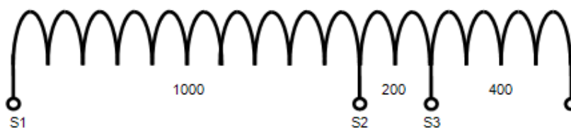
Figure 6: Tapping Arrangement for multi-ratio 1/1600T Buszone Cores
