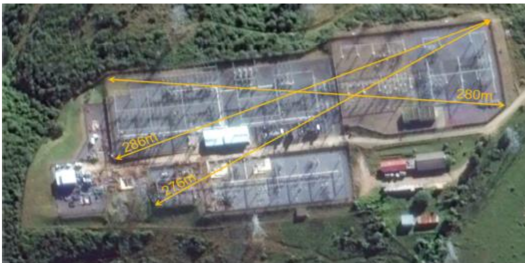
Figure 2: Determining current injection distance
