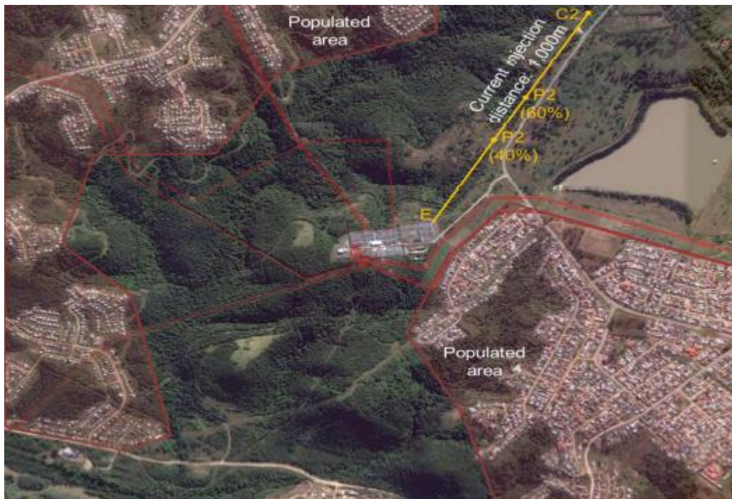
Figure 3: Determining current injection distance and area
