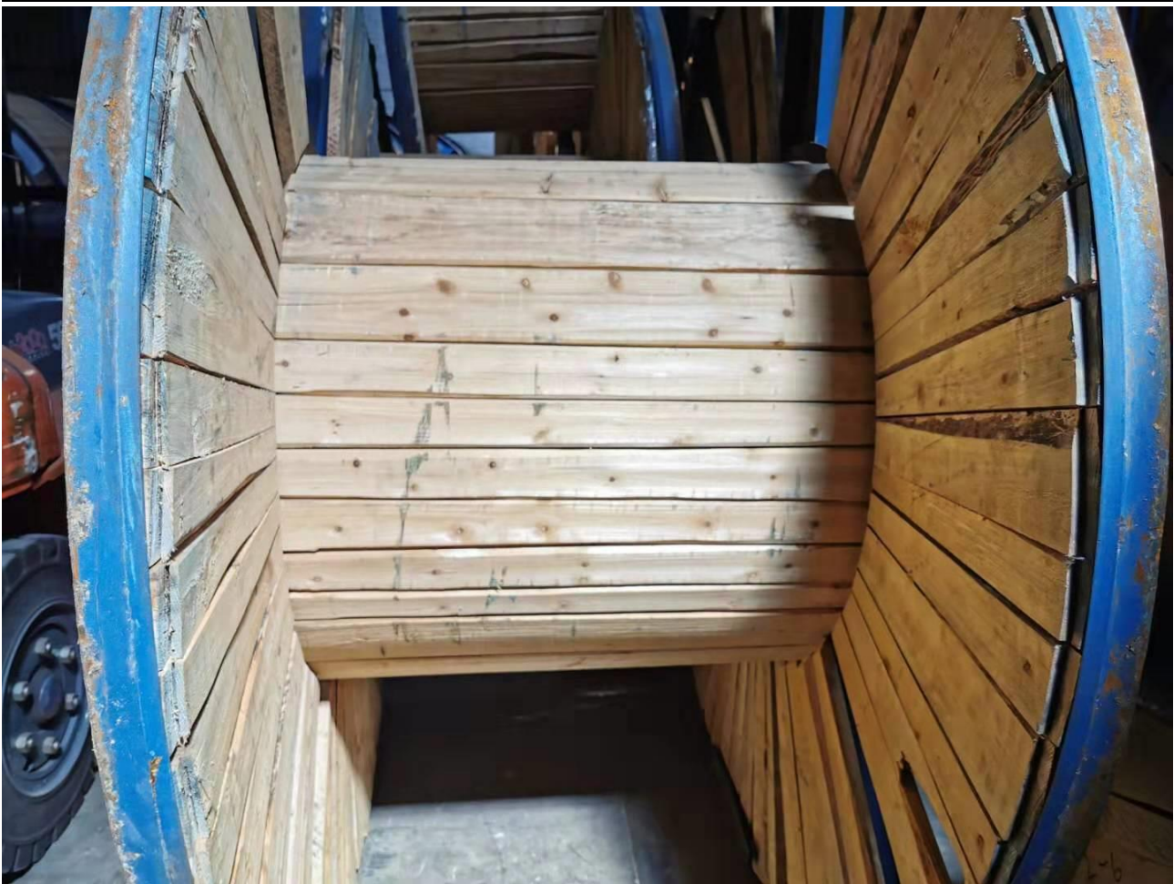
Figure 9-3 typical hybrid drum front view
