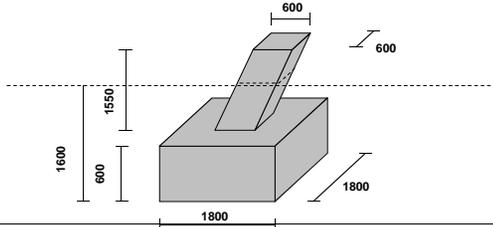
Soil Layer on top of pad assumed = 1000 mm
