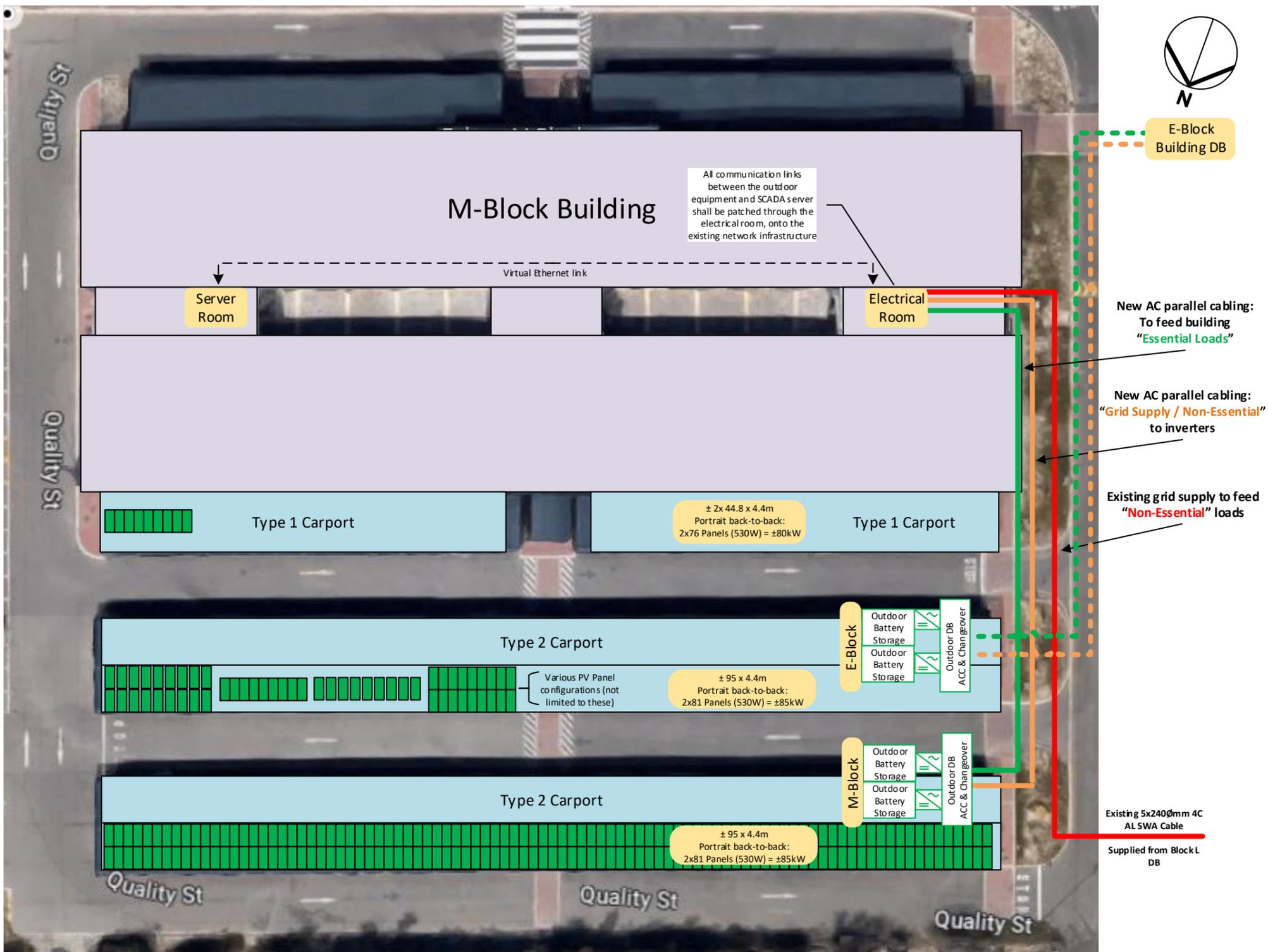
Figure 4 - Solar PV Site M-block Carport and proposed equipment layout and cabling
