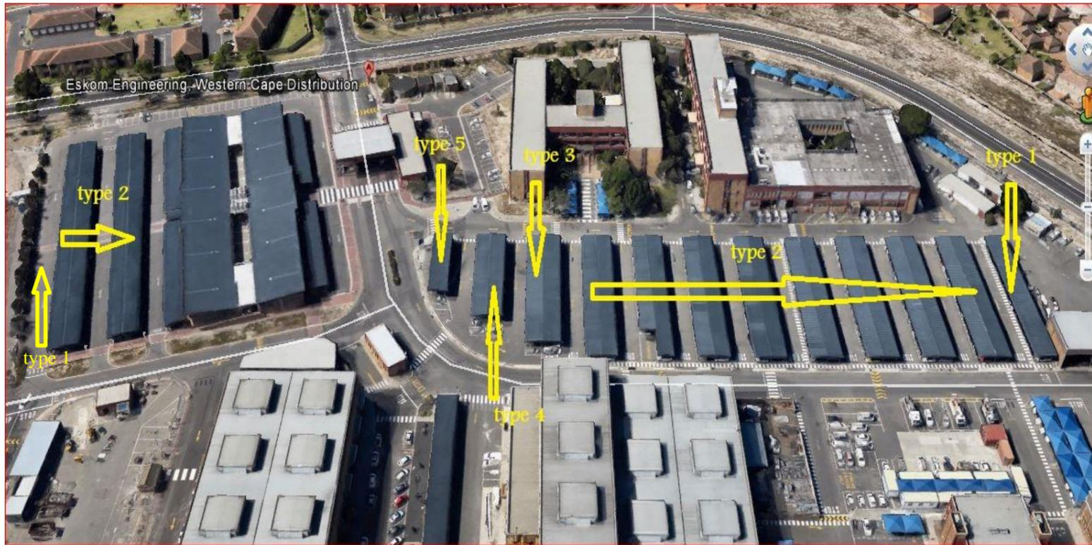
Figure 3 - Solar PV Site Carport Types
