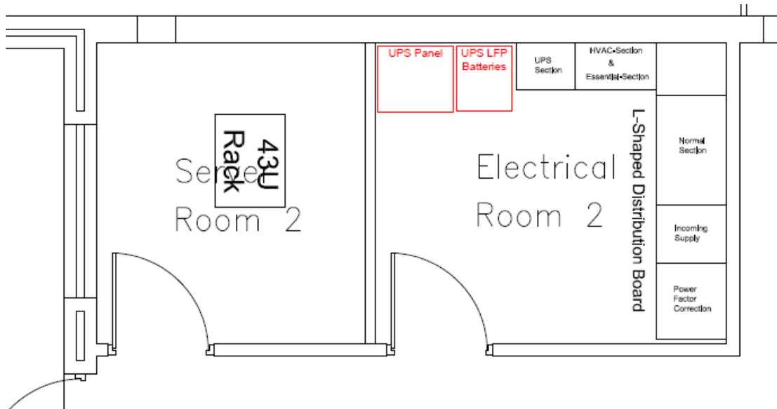
Figure 5 - M-Block building Main DB room
