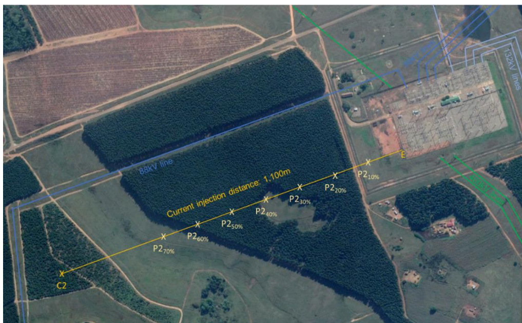
Figure 10: Determining current injection distance and direction
