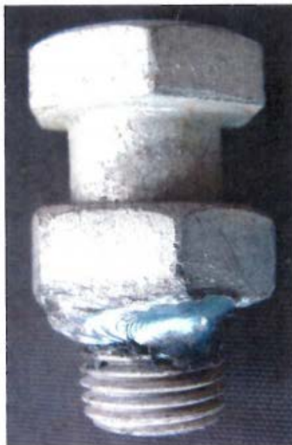
Photograph 1: Reveals the position of the weld
