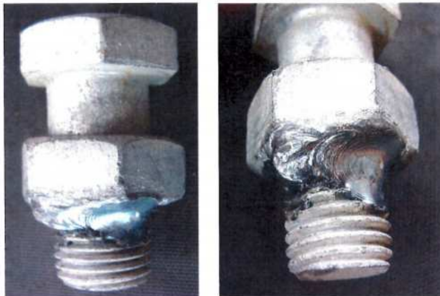
Photograph 1: Reveals the position of the weld
