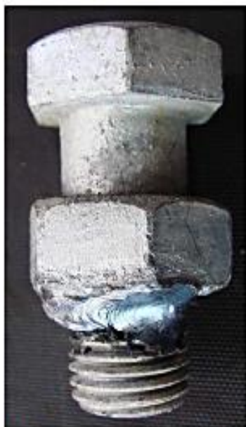
Photograph 1: Reveals the position of the weld
