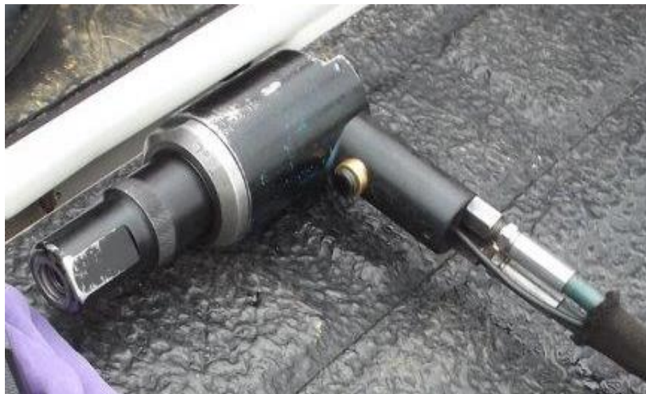
Figure A3: Hydraulic crimper with one side flatten
