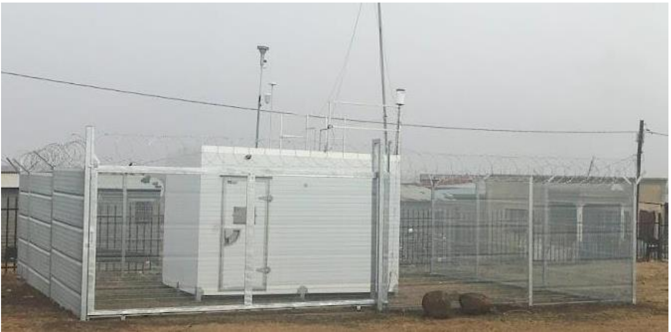
Figure 2: The reference ambient air quality monitoring station at Sivukile.
