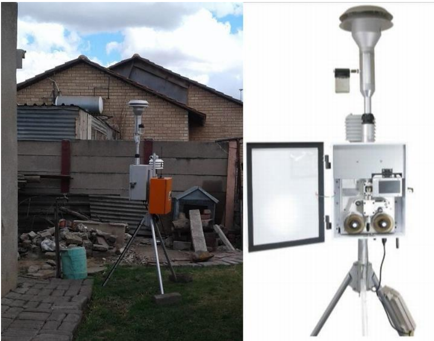
Figure 5: Portable Environmental Beta Attenuation Mass (E-BAM) Monitor
