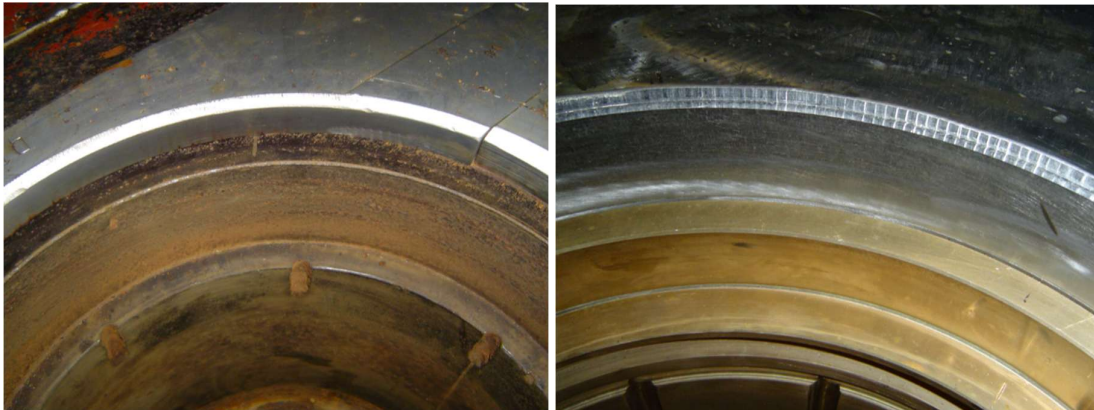
Figure 11.1.2: Bottom bush casing before and after repairs
