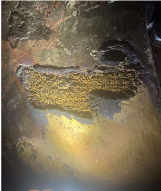
Figure 11.4.1: Draft tube liner damage (typical for spiral casing liner as well)
