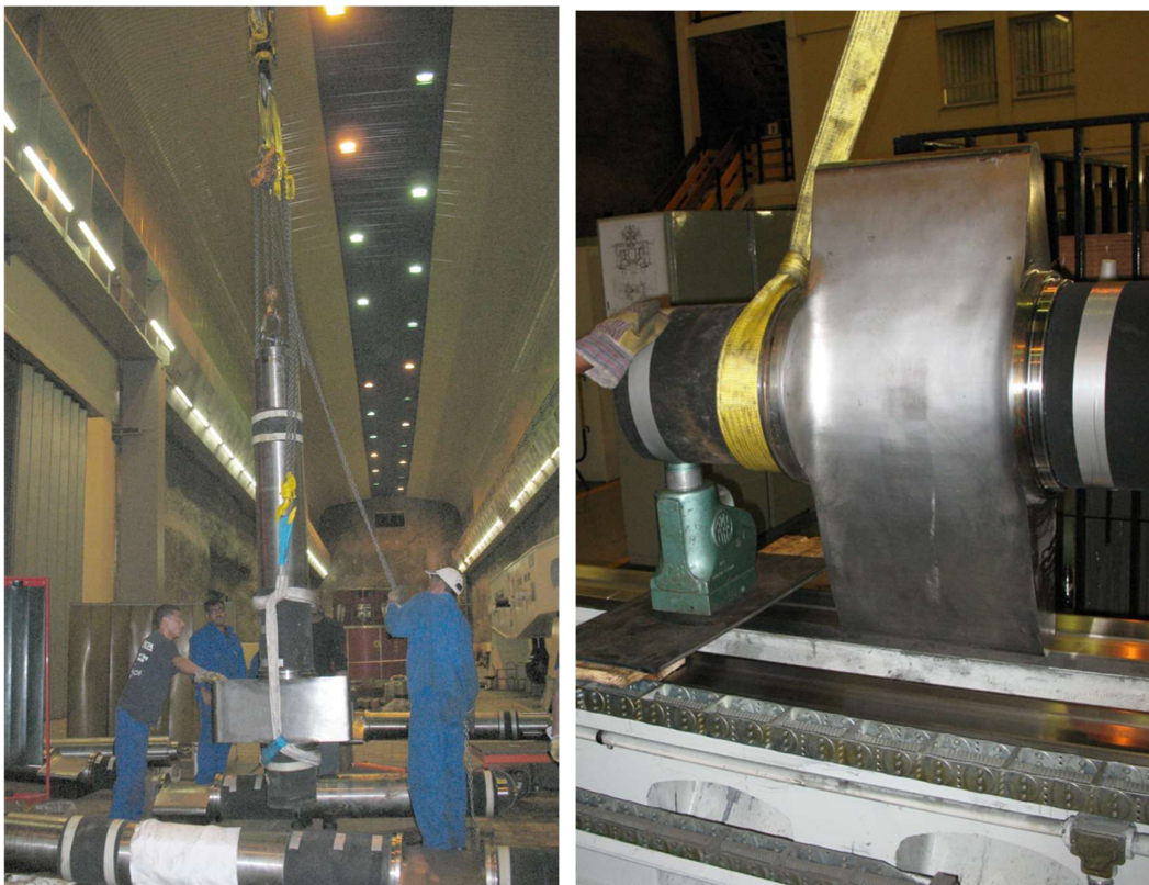
Figure11.8.2: Guide vane and guide vane blade
