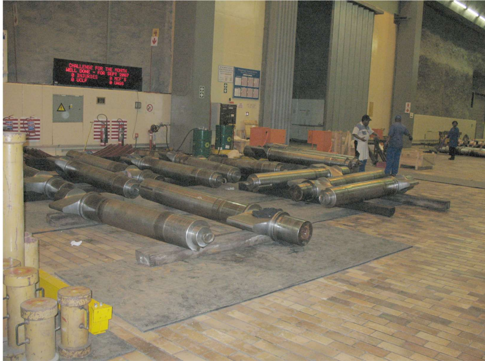
Figure 11.8.3: Guide vanes removed and placed on machine hall floor
