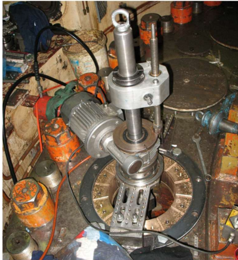
Figure 11.2.1: 2007 Guide vane top bush machining setup
