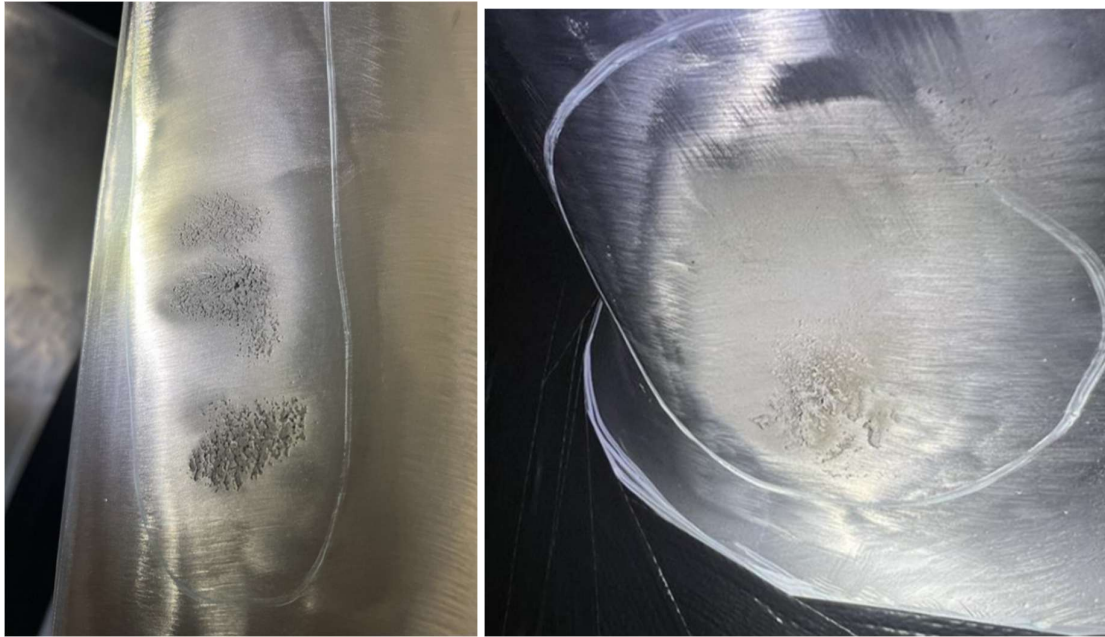
Figure11.10.1: Turbine runner blades cavitation and damage
