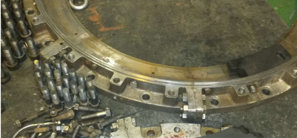
Figure 11.14.1: Shaft seal upper case housing O-ring groove damage_1
