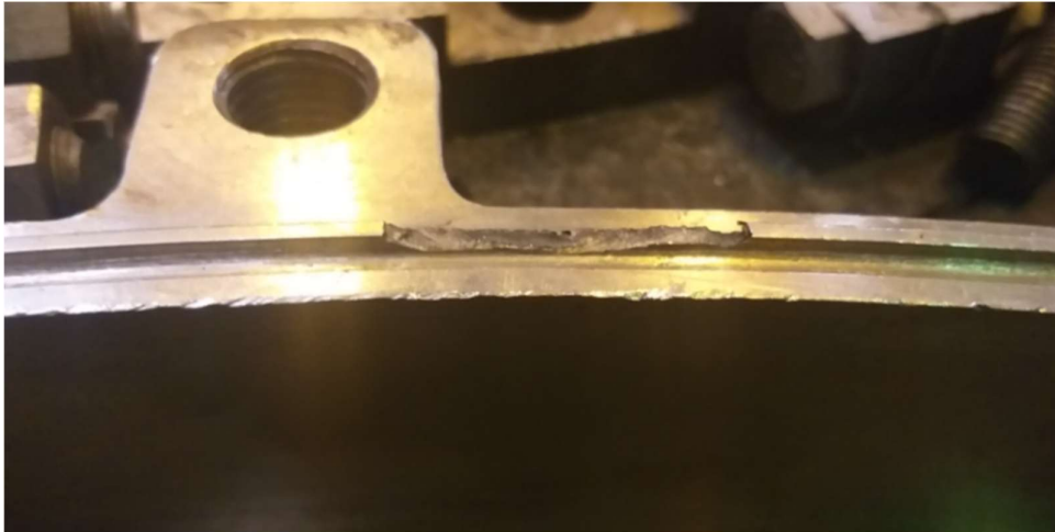
Figure 11.14.2: Shaft seal upper case housing O-ring groove damage_2
