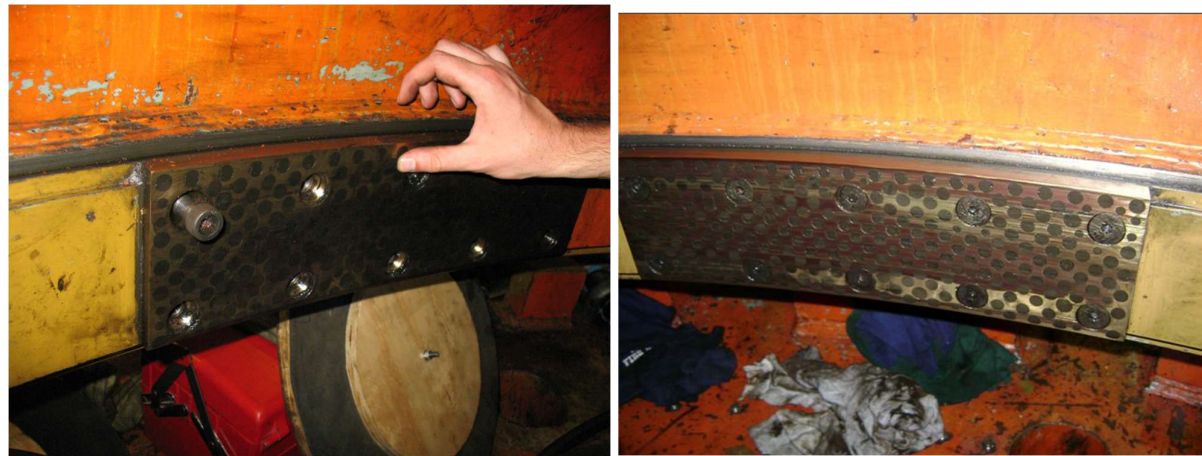
Figure 11.7.2: Vertical wear plate with flat rectangular locking plate on each side
