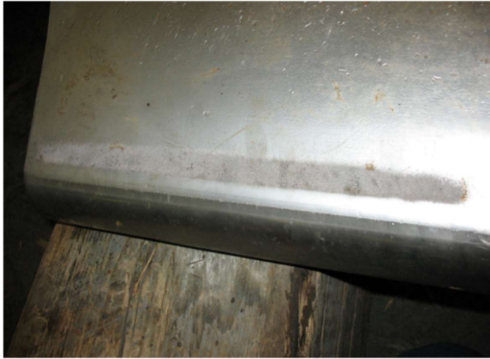
Figure 11.8.1: Example of dispersed guide vane cavitation
