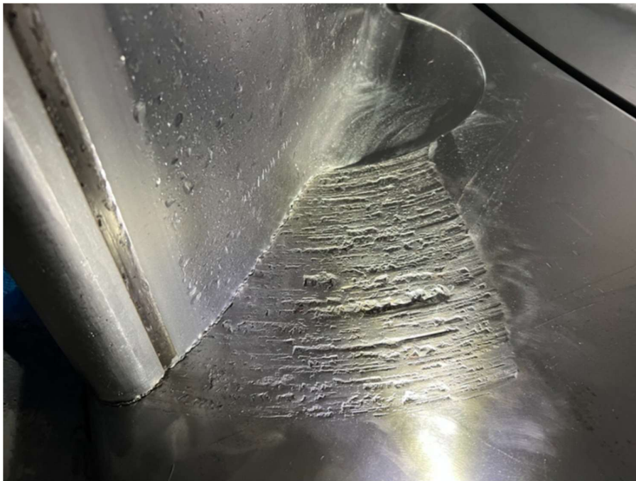
Figure 11.9.1: Guide vane facing plate previous pick-up removal by flapper disc
