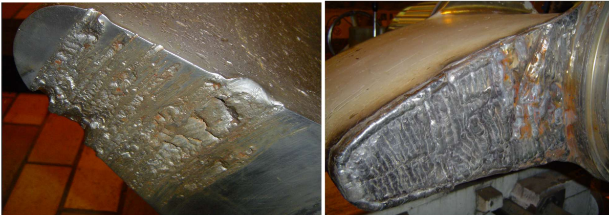
Figure 11.8.4: Guide vane upper and lower interfacing face repair welding prior to lathe machining
