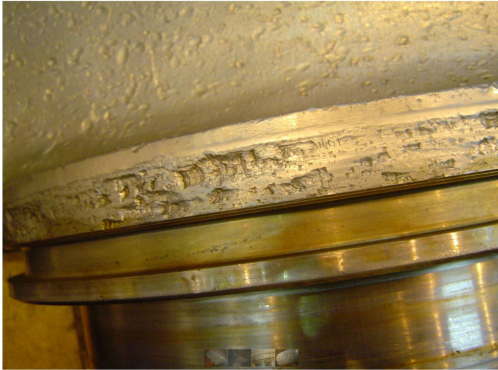
Figure 11.8.5: Guide vane collar damage
