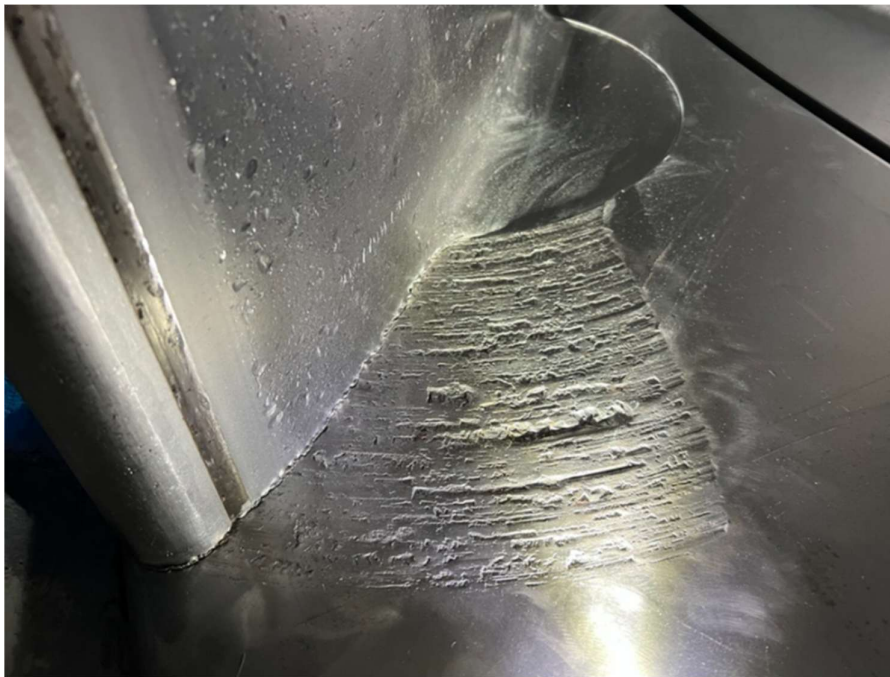
Figure 11.9.1: Guide vane facing plate previous pick-up removal by flapper disc
