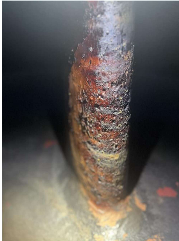
Figure 11.3.2: Example of damage on vertical stay vane
