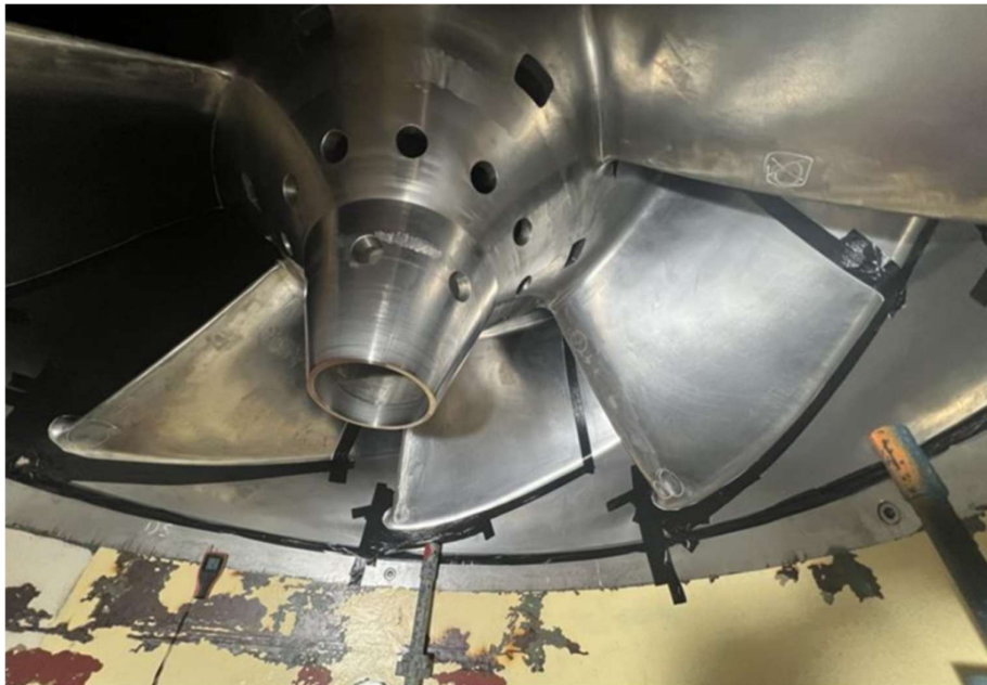
Figure 11.10.2: Bottom view of runner blades with marked cavitation areas
