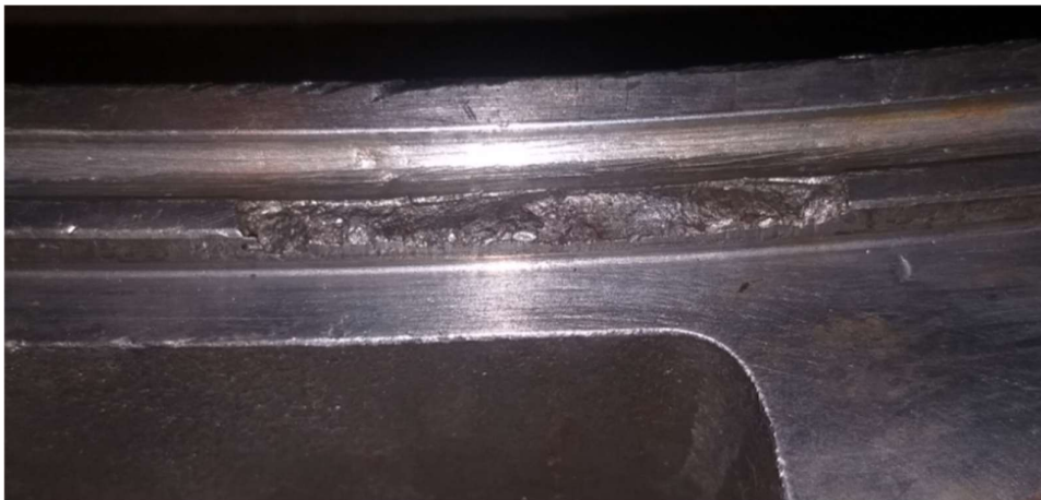
Figure 11.14.3: Shaft seal upper case housing O-ring groove damage_3
