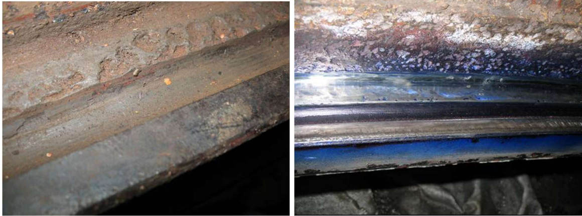
Figure 11.5.14: O-ring groove and surrounding surfaces' damage as per previous outages
