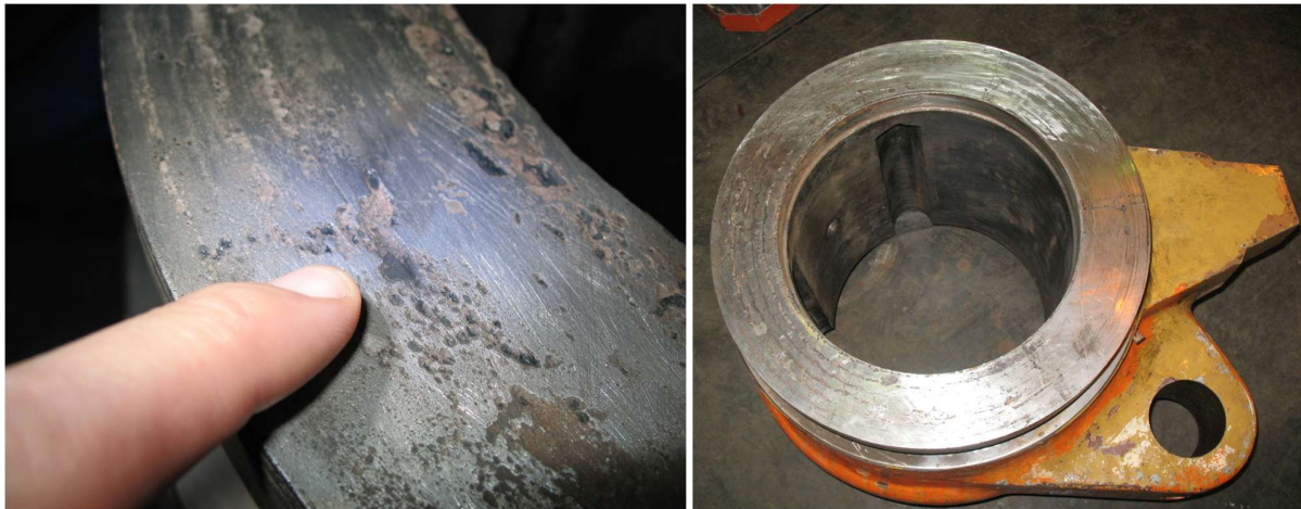
Figure11.11.3: Example of previous damage on guide vane head bottom flange surface
