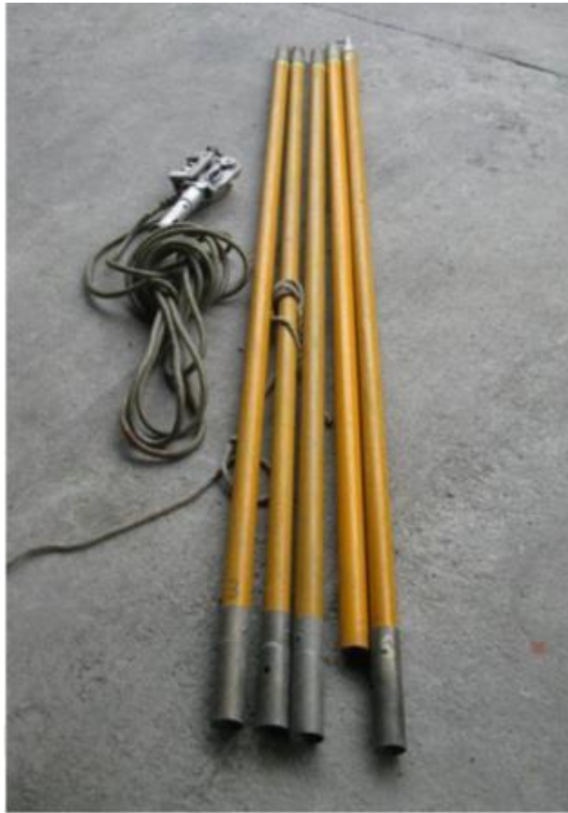
Figure C.1: Example of insulated earth sticks
